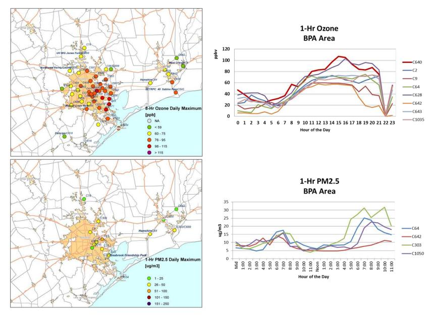
Figure 3-11. Regional ozone (top left and right) and PM<sub>2.5</sub> (bottom left and right) measurements (BPA area time series).
