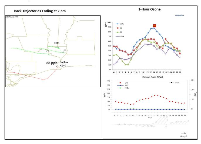
Figure 3-43. May 22, 2012 high ozone day at Sabine Pass C640. Left panel: AQPlot back trajectories ending at C640 and three background sites at the time of peak 1-hr ozone was observed at C640. Upper right panel: 1-hour average ozone time series for the C640 and background monitors. Lower right panel: time series of 1-hour ozone, NO, NO<sub>2</sub> and wind vectors at the Sabine Pass C640.
