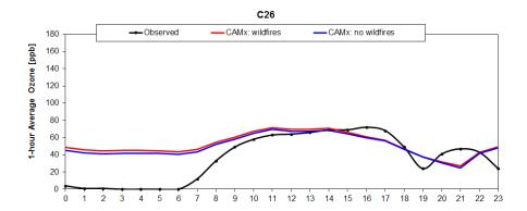
Figure 6-32. Northwest Harris County observed 1-hour ozone (black) versus modeled 1-hour average surface layer ozone for the CAMx run with fire emissions (red) and the CAMx run with no fire emissions (blue).
