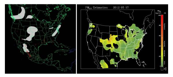
Figure 3-30. Left panel: HMS product showing May 17 fire locations (red dots) and smoke plume (gray area). Right panel: IDEA surface PM<sub>2.5</sub> estimate based on AOD and surface monitoring data.
