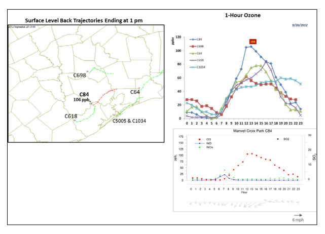
Figure 3-104. September 20, 2012 high ozone day at Manvel Croix C84. Left panel: AQPlot back trajectories ending at C84 and four background sites at the time of peak 1-hr ozone was observed at C84. Upper right panel: 1-hour average ozone time series for the CAMS84 and background monitors. Lower right panel: time series of 1-hour ozone, NO, NO<sub>2</sub> and wind vectors at the Manvel Croix C84.
