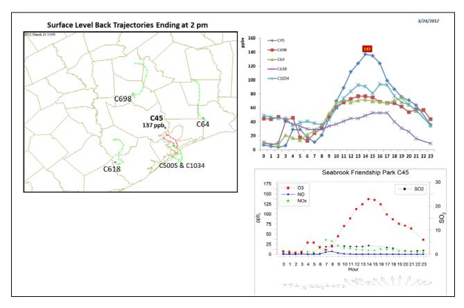
Figure 3-3. March 24, 2012 high ozone day at Seabrook Friendship Park C45. Left panel: AQPlot back trajectories terminating at C45 and four HGB monitors located outside the central urban area at the time of peak 1-hour ozone at C45. Upper right panel: 1-hour average ozone time series for C45 and surrounding HGB monitors. Lower right panel: time series of 1-hour ozone, NO, NO<sub>2</sub>, SO<sub>2</sub> and wind vectors at the Seabrook Friendship Park C45 monitor on March 24.
