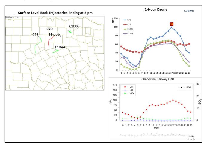
Figure 3-59. June 24, 2012 high ozone day at Grapevine Fairway C70. Left panel: AQPlot back trajectories ending at C70 and four background sites at the time of peak 1-hr ozone was observed. Upper right panel: 1-hour average ozone time series for the C70 and background monitors. Lower right panel: time series of 1-hour ozone, NO, NO<sub>2</sub> and wind vectors at the Grapevine Fairway C70 site.
