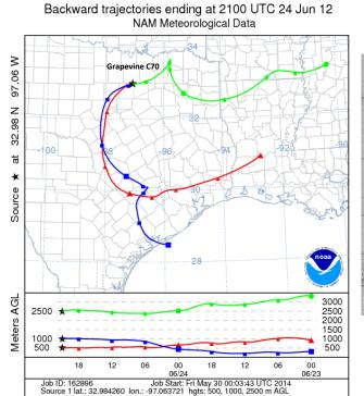
Trajectory Direction: Backward Duration: 72 hrs Vertical Motion Calculation Method: Model Vertical Velocity Meteorology: 0000Z 24 Jun 2012 - NAM12
