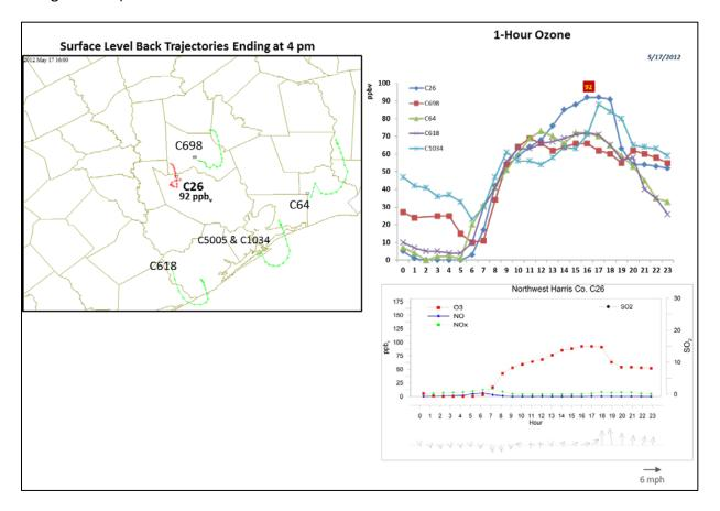
Figure 3-27. May 17, 2012 high ozone day at Northwest Harris Co. C26. Left panel: back trajectories calculated using AQPlot for the HGB monitors at the time of peak ozone impact at C26. Upper right panel: 1-hour average ozone time series for the C26 and surrounding HGB monitors. Lower right panel: time series of 1-hour ozone, NO, NO<sub>2</sub> and wind vectors at the Northwest Harris monitor.
