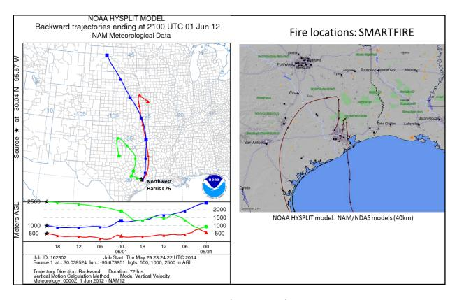
Figure 3-51. 72-hour HYSPLIT back trajectories (NAM 12km) from Northwest Harris C26 ending June 1, 2012; SmartFire plot showing fire locations (orange triangles) and 72-hour HYSPLIT back trajectories (EDAS 40 km) from C26.
