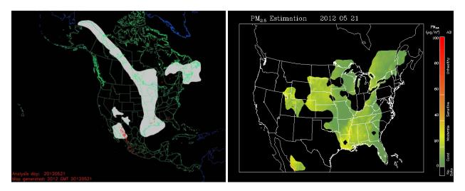
Figure 2-8. Left panel: HMS product showing fire locations (red dots) and smoke plume (gray area). Right panel: IDEA surface PM<sub>2.5</sub> estimate based on AOD and surface monitoring data.
