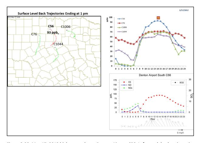
Figure 3-28. May 17, 2012 high ozone day at Denton Airport C56. Left panel: back trajectories calculated using AQPlot for the DFW monitors at the time of peak ozone impact at C56. Upper right panel: 1-hour average ozone time series for the C56 and surrounding DFW monitors. Lower right panel: time series of 1-hour ozone, NO, NO<sub>2</sub> and wind vectors at the Denton Airport C56.
