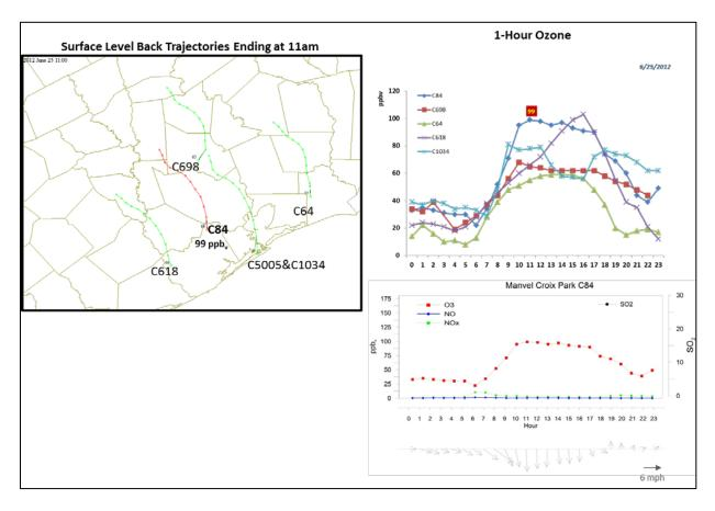
Figure 3-68. June 25, 2012 high ozone day at Manvel Croix Park C84. Left panel: AQPlot back trajectories ending at C84 and four background sites at the time of peak 1-hr ozone was observed. Upper right panel: 1-hour average ozone time series for the C84 and background monitors. Lower right panel: time series of 1-hour ozone, NO, NO<sub>2</sub> and wind vectors at the Grapevine Fairway C84 site.
