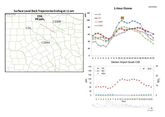
Figure 3-89. June 27, 2012 high ozone day at Denton Airport South C56. Left panel: AQPlot back trajectories ending at C56 and four background sites at the time of peak 1-hr ozone was observed. Upper right panel: 1-hour average ozone time series for the C70 and background monitors. Lower right panel: time series of 1-hour ozone, NO, NO<sub>2</sub> and wind vectors at the Grapevine Fairway C56 site.
