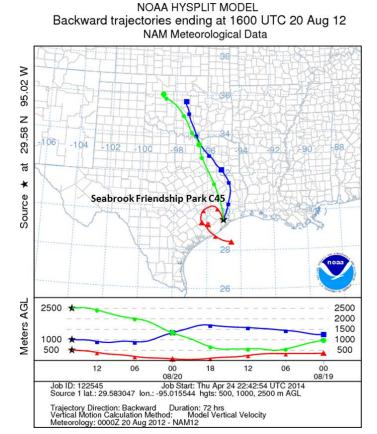
Figure 2-6. HYSPLIT back trajectories terminating at Seabrook Friendship Park C45. Back trajectories are shown for three altitudes (500 m, 1,500 m and 2,500 m) using NAM 12km meteorology.
