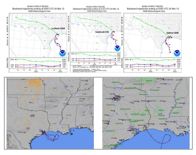
Figure 3-6. March 24 72-hour HYSPLIT back trajectories at La Porte (top left); Seabrook (top middle) and Sabine site (top right); SmartFire plots showing fire locations for March 24 (orange triangles) and 72-hour back trajectories from HGB sites (bottom left) and BPA Sabine C640 site location (bottom right).
