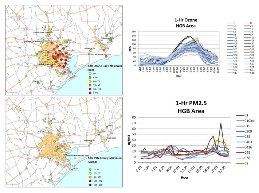
Figure 3-12. Regional ozone (top left and right) and PM<sub>2.5</sub> (bottom left and right) measurements (HGB area time series).
