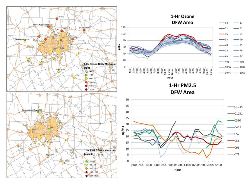
Figure 3-96. Regional ozone (top left and right) and PM<sub>2.5</sub> (bottom left and right) measurements (DFW area time series).
