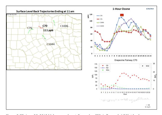
Figure 3-77. June 26, 2012 high ozone day at Grapevine C70. Left panel: AQPlot back trajectories ending at C70 and four background sites at the time of peak 1-hr ozone was observed. Upper right panel: 1-hour average ozone time series for the C70 and background monitors. Lower right panel: time series of 1-hour ozone, NO, NO<sub>2</sub> and wind vectors at the Grapevine Fairway C70 site.
