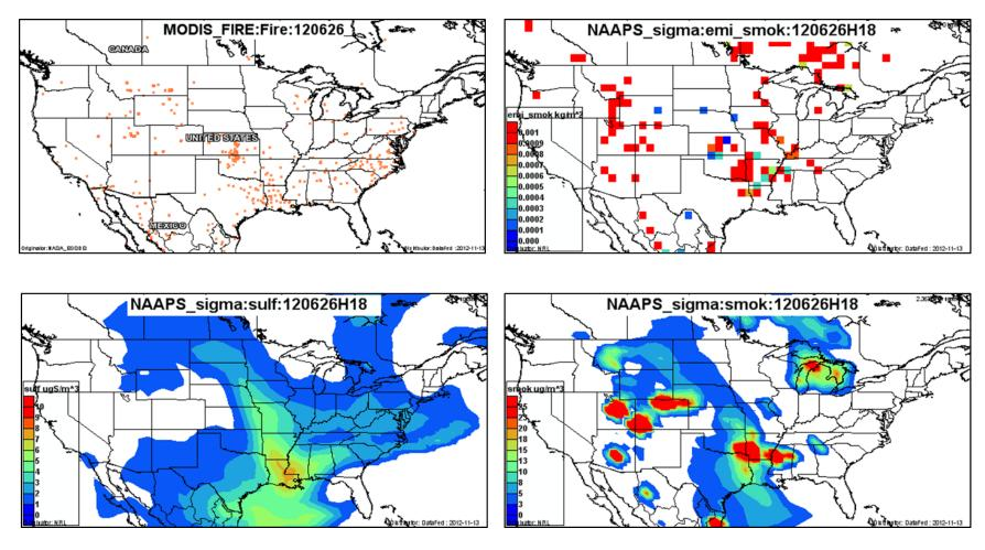
Figure 3-83. June 26, 2012 DataFed analysis. Upper left panel: Locations of active fires from MODIS satellite fire detections. Upper right panel: NAAPS model smoke emissions. Lower left panel: NAAPS model surface layer sulfate concentrations. Lower right panel: NAAPS model surface layer smoke concentrations.
