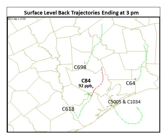
Figure 2-1. July 2, 2013 AQPlot surface wind back trajectories terminating at HGB area ozone monitoring sites outside or on the periphery of the HGB urban area.
