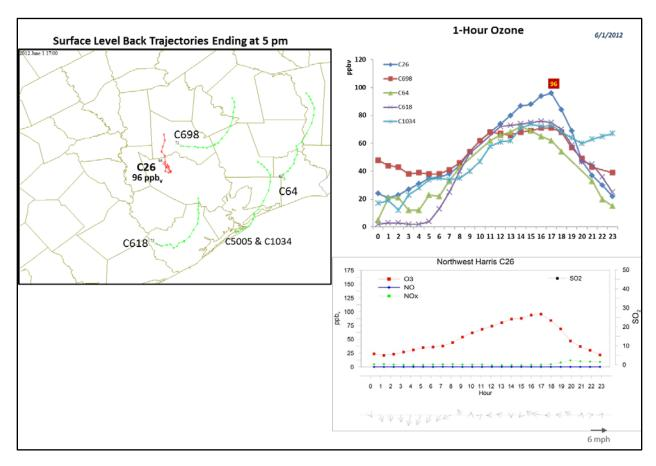
Figure 3-50. June 1, 2012 high ozone day at Northwest Harris C26. Left panel: AQPlot back trajectories ending at C26 and four background sites at the time of peak 1-hr ozone was observed at C26. Upper right panel: 1-hour average ozone time series for the C26 and background monitors. Lower right panel: time series of 1-hour ozone, NO, NO<sub>2</sub> and wind vectors at the Northwest Harris C26.
