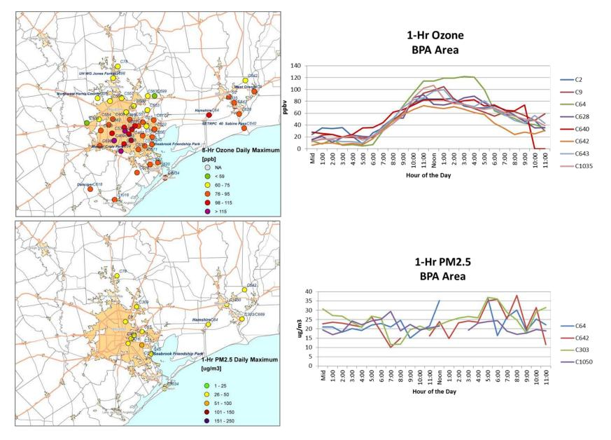
Figure 3-85. Regional ozone (top left and right) and PM<sub>2.5</sub> (bottom left and right) measurements (BPA area time series).
