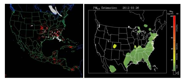
Figure 3-22. Left panel: HMS product showing March 26 fire locations (red dots) and smoke plume (gray area). Right panel: IDEA surface PM<sub>2.5</sub> estimate based on AOD and surface monitoring data.
