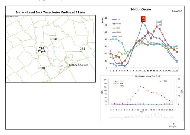
Figure 3-87. June 27, 2012 high ozone day at Northwest Harris C26. Left panel: AQPlot back trajectories ending at C26 and four background sites at the time of peak 1-hr ozone was observed. Upper right panel: 1-hour average ozone time series for the C26 and background
