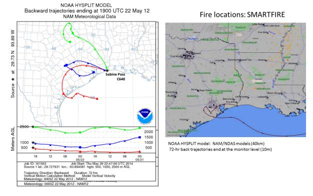
Figure 3-44. 72-hour HYSPLIT back trajectories (NAM 12km) from Sabine Pass C640 ending May 22, 2012; SmartFire plot showing fire locations (orange triangles) and 72-hour HYSPLIT back trajectories (EDAS 40 km) from C640.
