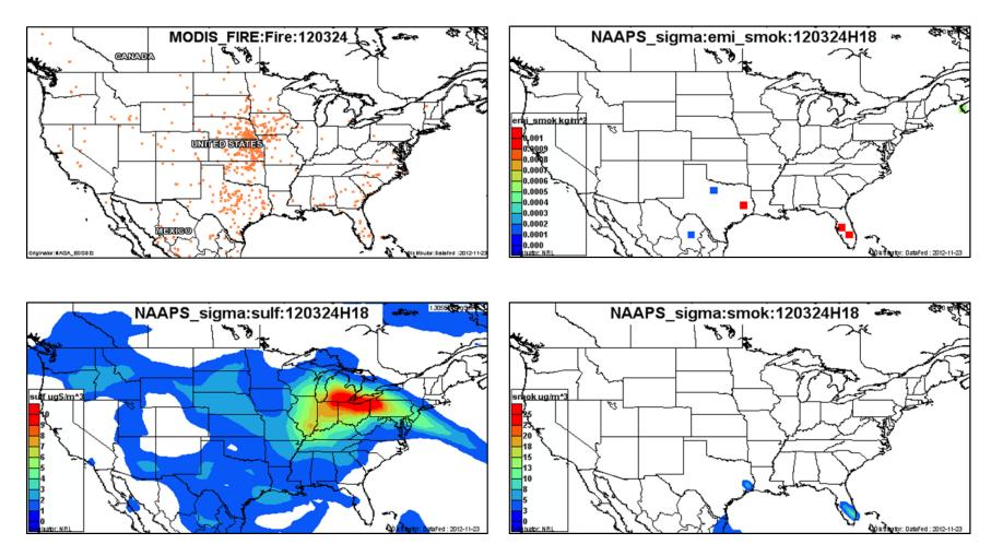
Figure 3-10. March 24, 2012 DataFed analysis. Upper left panel: Locations of active fires from MODIS satellite fire detections. Upper right panel: NAAPS model smoke emissions. Lower left panel: NAAPS model surface layer sulfate concentrations. Lower right panel: NAAPS model surface layer smoke concentrations.
