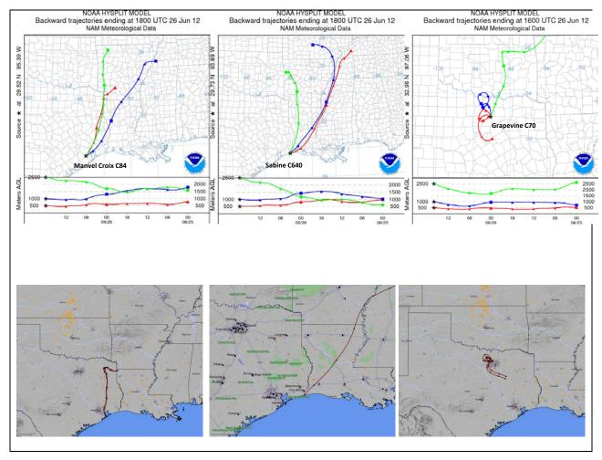
Figure 3-79. 72-hour HYSPLIT back trajectories at Manvel Croix C84 (top left); Sabine Pass C640 (middle) and Grapevine Fairway C70 (top right); SmartFire plots showing fire locations (orange triangles) and 72-hour HYSPLIT back trajectories from HGB (bottom left) and BPA area (bottom center) and DFW (bottom right)
