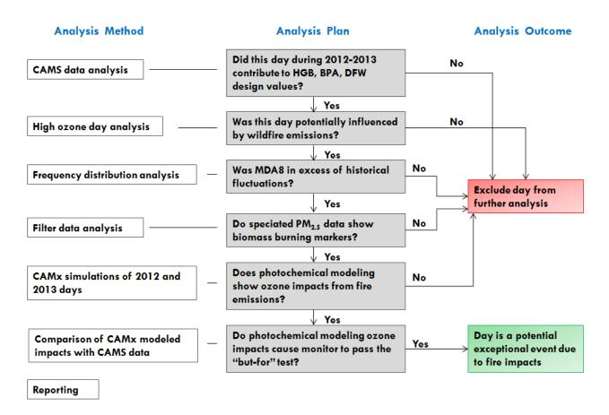
Figure 1-1. Summary of method for determining whether high ozone days meet the four EER criteria.
