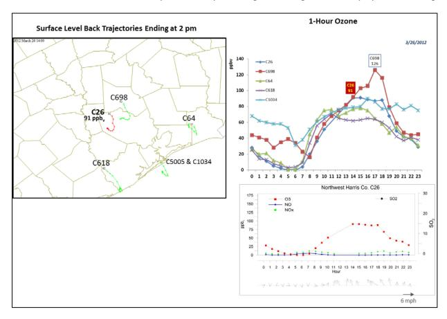
Figure 3-20. March 26, 2012 high ozone day at Northwest Harris County, C26. Left panel: back trajectories from AQPlot for the HGB monitors for March 26 at the time of peak 1-hour ozone at C26. Upper right panel: 1-hour average ozone time series for the C26 and surrounding HGB monitors. Lower right panel: time series of 1-hour ozone, NO, NO<sub>2</sub> and wind vectors at the Northwest Harris monitor on March 26.
