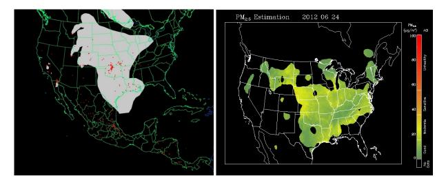
Figure 3-61. Left panel: HMS product showing June 24 fire locations (red dots) and smoke plume (gray area). Right panel: IDEA surface PM<sub>2.5</sub> estimate based on AOD and surface monitoring data.
