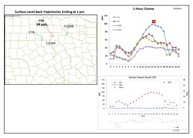
Figure 3-97. September 6, 2012 high ozone day at Denton Airport C56. Left panel: AQPlot back trajectories ending at C56 and four background sites at the time of peak 1-hr ozone was observed. Upper right panel: 1-hour average ozone time series for the C56 and background monitors. Lower right panel: time series of 1-hour ozone, NO, NO<sub>2</sub> and wind vectors at Denton C56 site.
