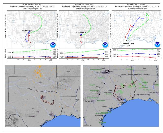
Figure 3-69. 72-hour HYSPLIT back trajectories at Denton C56 (top left); Grapevine C70 (middle) and Manvel Croix C84 (top right); SMARTFIRE plots showing fire locations (orange triangles) and 72-hour HYSPLIT back trajectories from DFW sites (bottom left) and HGB area (bottom right).
