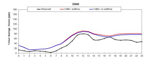
Figure 6-36. Sabine Pass observed 1-hour ozone (black) versus modeled 1-hour average surface layer ozone for the CAMx run with fire emissions (red) and the CAMx run with no fire emissions (blue).
