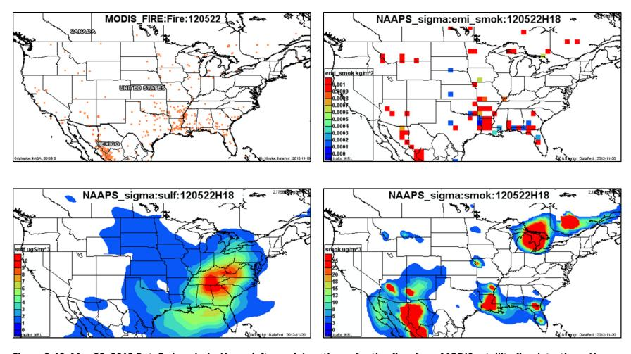
Figure 3-48. May 22, 2012 DataFed analysis. Upper left panel: Locations of active fires from MODIS satellite fire detections. Upper right panel: NAAPS model smoke emissions. Lower left panel: NAAPS model surface layer sulfate concentrations. Lower right panel: NAAPS model surface layer smoke concentrations.
