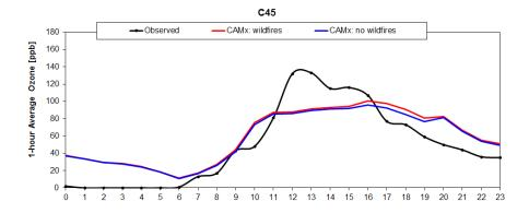
Figure 6-34. Seabrook observed 1-hour ozone (black) versus modeled 1-hour average surface layer ozone for the CAMx run with fire emissions (red) and the CAMx run with no fire emissions (blue).
