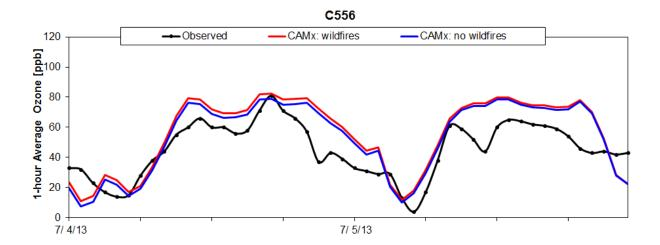
Figure 6-28. La Porte observed 1-hour ozone (black) versus modeled 1-hour average surface layer ozone for the CAMx run with fire emissions (red) and the CAMx run with no fire emissions (blue).
