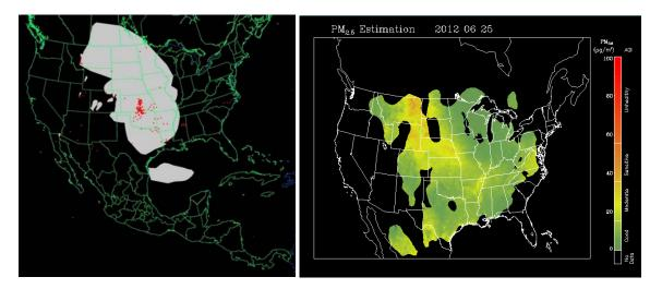
Figure 3-70. Left panel: HMS product showing June 25 fire locations (red dots) and smoke plume (gray area). Right panel: IDEA surface PM<sub>2.5</sub> estimate based on AOD and surface monitoring data.
