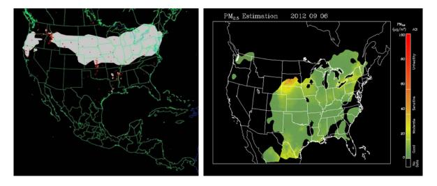
Figure 3-99. Left panel: HMS product showing September 6 fire locations (red dots) and smoke plume (gray area). Right panel: IDEA surface PM<sub>2.5</sub> estimate based on AOD and surface monitoring data.
