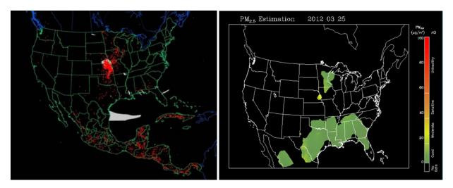
Figure 3-15. Left panel: HMS product showing March 25 fire locations (red dots) and smoke plume (gray area). Right panel: IDEA surface PM<sub>2.5</sub> estimate based on AOD and surface monitoring data.
