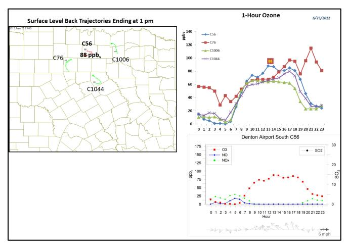
Figure 3-66. June 25, 2012 high ozone day at Denton Airport South C56. Left panel: AQPlot back trajectories ending at C56 and four background sites at the time of peak 1-hr ozone was observed. Upper right panel: 1-hour average ozone time series for the C70 and background monitors. Lower right panel: time series of 1-hour ozone, NO, NO<sub>2</sub> and wind vectors at the Grapevine Fairway C56 site.
