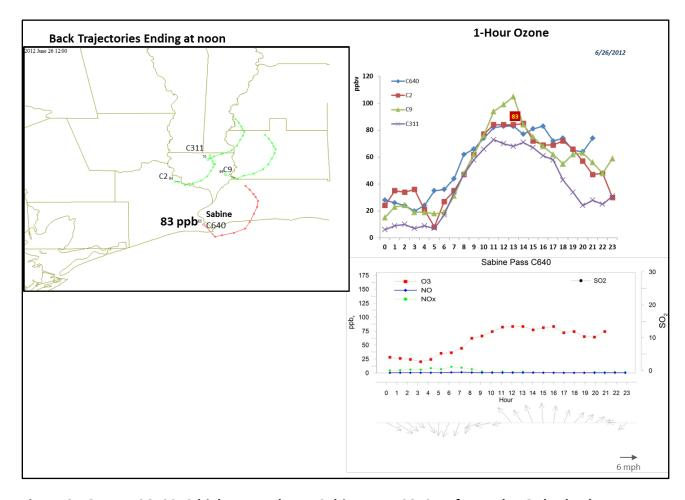
Figure 3-78. June 26, 2012 high ozone day at Sabine Pass C640. Left panel: AQPlot back trajectories ending at C640 and four background sites at the time of peak 1-hr ozone was observed. Upper right panel: 1-hour average ozone time series for the C640 and background monitors. Lower right panel: time series of 1-hour ozone, NO, NO<sub>2</sub> and wind vectors at the Sabine Pass C640 site.
