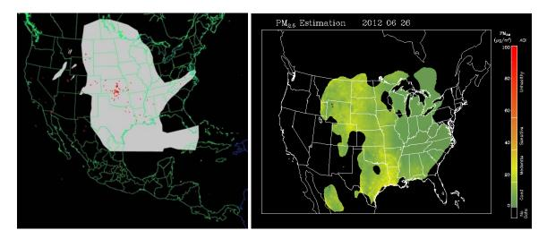
Figure 3-80. Left panel: HMS product showing June 26 fire locations (red dots) and smoke plume (gray area). Right panel: IDEA surface PM<sub>2.5</sub> estimate based on AOD and surface monitoring data.
