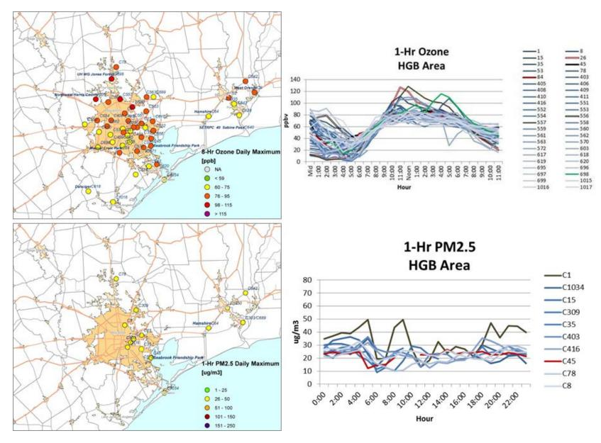
Figure 3-95. Regional ozone (top left and right) and PM2.5 (bottom left and right) measurements (HGB area time series).
