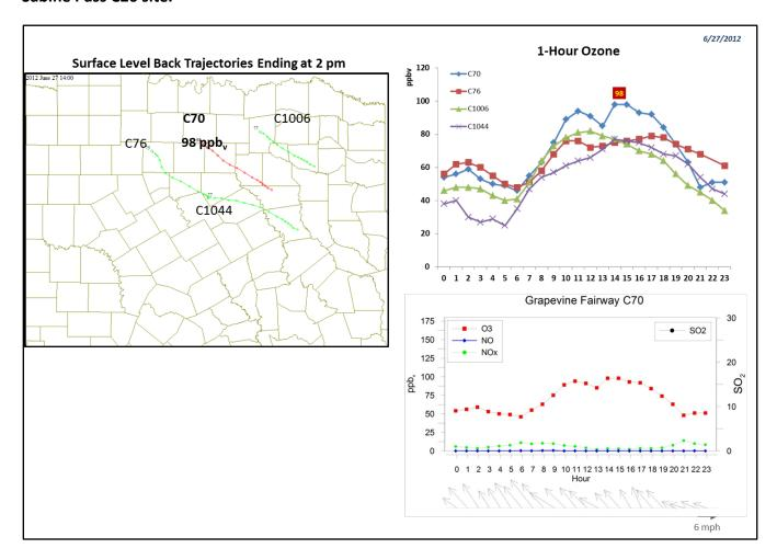
Figure 3-88. June 27, 2012 high ozone day at Grapevine Fairway C70. Left panel: AQPlot back trajectories ending at C70 and four background sites at the time of peak 1-hr ozone was observed. Upper right panel: 1-hour average ozone time series for the C70 and background monitors. Lower right panel: time series of 1-hour ozone, NO, NO<sub>2</sub> and wind vectors at the Grapevine C70 site.
