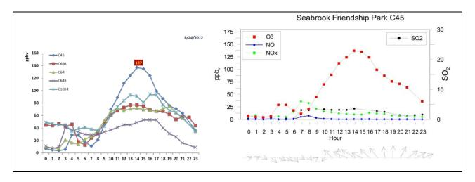
Figure 2-2. Ambient measurements at the Seabrook Friendship Park C45 with background sites (left) coupled with ozone, NO, NOx, SO<sub>2</sub> and wind vectors (right).
