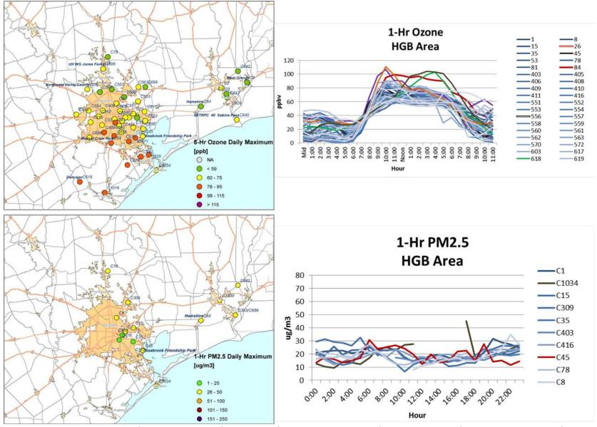
Figure 3-74. Regional ozone (top left and right) and PM<sub>2.5</sub> (bottom left and right) measurements (HGB area time series).
