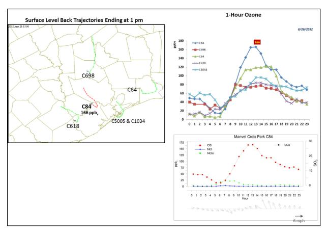
Figure 3-76. June 26, 2012 high ozone day at Manvel Croix Park C84. Left panel: AQPlot back trajectories ending at C84 and four background sites at the time of peak 1-hr ozone was observed. Upper right panel: 1-hour average ozone time series for the C84 and background monitors. Lower right panel: time series of 1-hour ozone, NO, NO<sub>2</sub> and wind vectors at the Manvel Croix Park C84 site.
