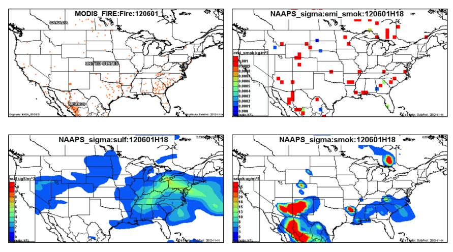
Figure 3-55. June 1, 2012 DataFed analysis. Upper left panel: Locations of active fires from MODIS satellite fire detections. Upper right panel: NAAPS model smoke emissions. Lower left panel: NAAPS model surface layer sulfate concentrations. Lower right panel: NAAPS model surface layer smoke concentrations.
