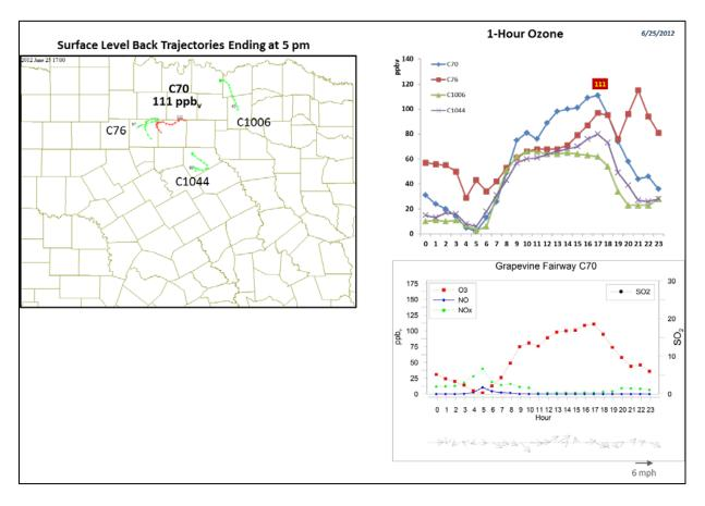
Figure 3-67. June 25, 2012 high ozone day at Grapevine Fairway C70. Left panel: AQPlot back trajectories ending at C70 and four background sites at the time of peak 1-hr ozone was observed. Upper right panel: 1-hour average ozone time series for the C70 and background monitors. Lower right panel: time series of 1-hour ozone, NO, NO<sub>2</sub> and wind vectors at the Grapevine Fairway C70 site.
