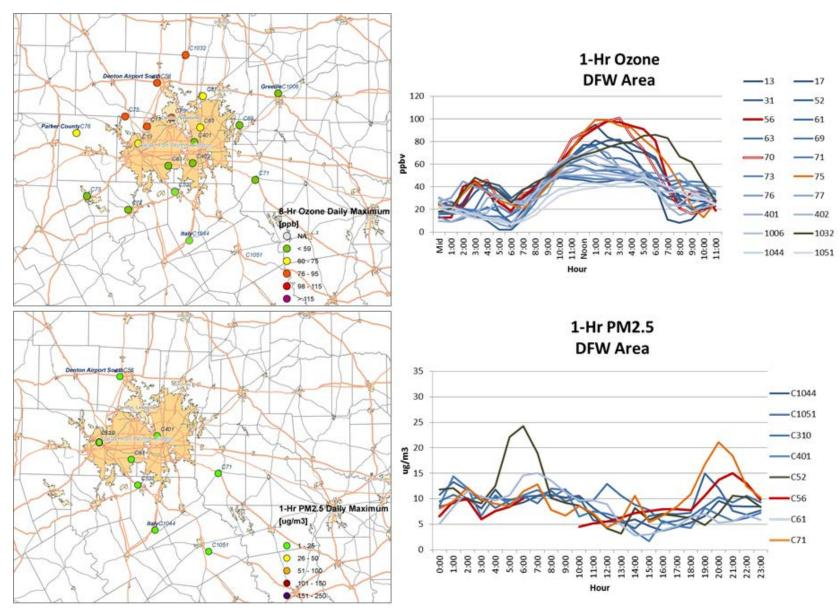
Figure 3-103. Regional ozone (top left and right) and PM<sub>2.5</sub> (bottom left and right) measurements (DFW area time series).
