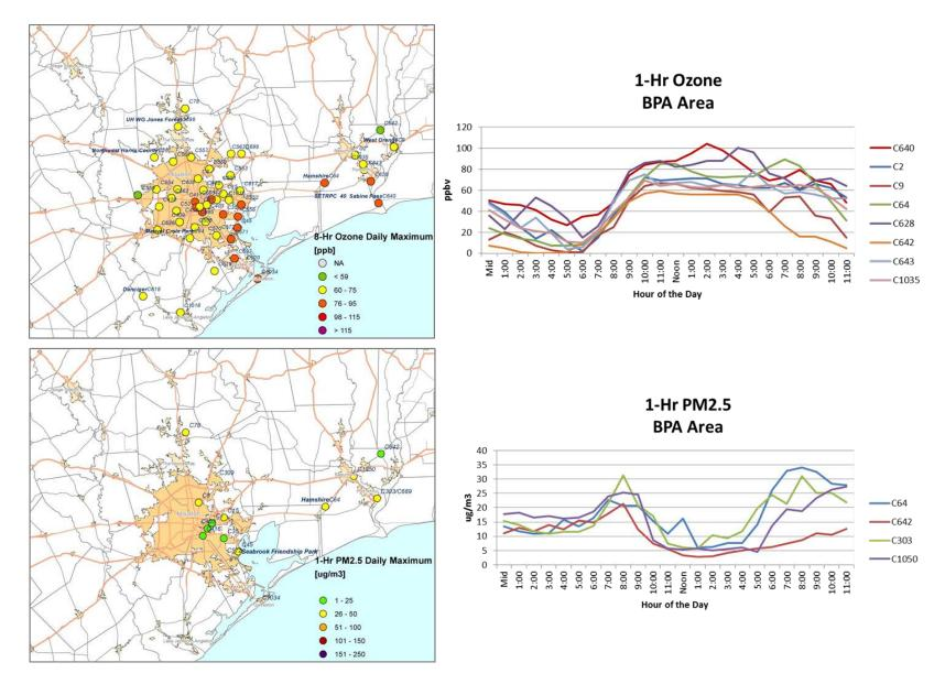
Figure 3-19. March 25 Regional ozone (top left and right) and PM<sub>2.5</sub> (bottom left and right) measurements (BPA area time series.
