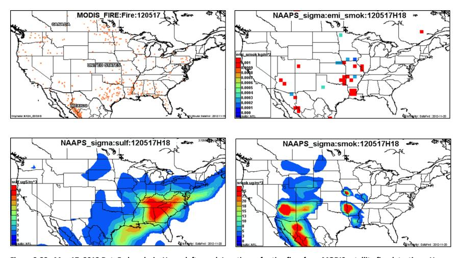
Figure 3-33. May 17, 2012 DataFed analysis. Upper left panel: Locations of active fires from MODIS satellite fire detections. Upper right panel: NAAPS model smoke emissions. Lower left panel: NAAPS model surface layer sulfate concentrations. Lower right panel: NAAPS model surface layer smoke concentrations.
