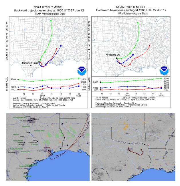
Figure 3-90. 72-hour HYSPLIT back trajectories at Northwest Harris C26 (top left); Grapevine C70 (right); SmartFire plots showing fire locations (orange triangles) and 72-hour HYSPLIT back trajectories from HGB area (bottom left) and DFW area monitors (bottom right).
