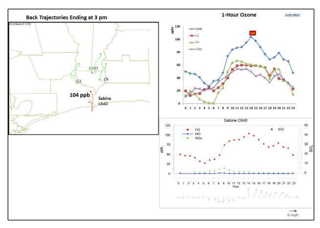
Figure 3-13. March 25, 2012 high ozone day at Sabine Pass C640. Left panel: back trajectories from AQPlot for 3 monitors located outside the central urban area at the time of peak 1-hour ozone at C640. Upper right panel: 1-hour average ozone time series for the C640 and surrounding BPA monitors. Lower right panel: time series of 1-hour ozone, NO, NO<sub>2</sub> and wind vectors at the Sabine monitor on March 25.
