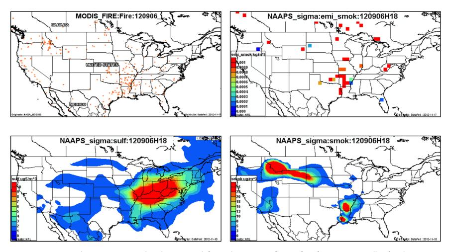
Figure 3-102. September 6, 2012 DataFed analysis. Upper left panel: Locations of active fires from MODIS satellite fire detections. Upper right panel: NAAPS model smoke emissions. Lower left panel: NAAPS model surface layer sulfate concentrations. Lower right panel: NAAPS model surface layer smoke concentrations.
