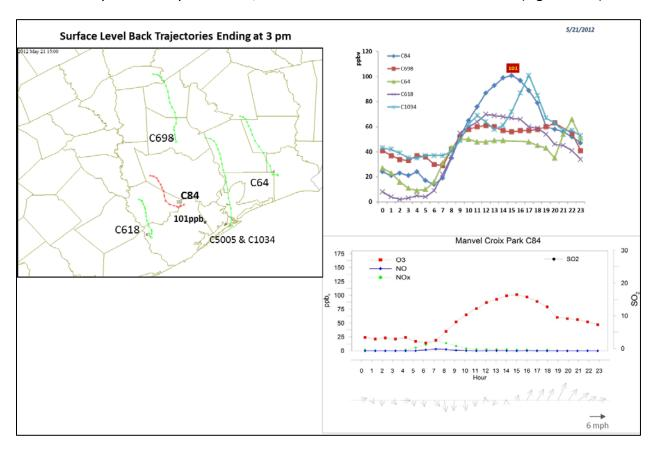
Figure 3-36. May 21, 2012 high ozone day at Manvel Croix Park C84. Left panel: back trajectories from C84 and background HGB monitors at the time of peak 1-hr ozone impact at C84. Upper right panel: 1-hour average ozone time series for the C84 and background monitors. Lower right panel: time series of 1-hour ozone, NO, NO<sub>2</sub> and wind vectors at the Manvel Croix Park. SO<sub>2</sub> is not monitored at the Manvel Croix CAMS.
