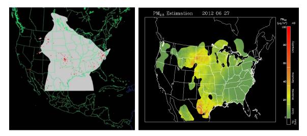
Figure 3-91. Left panel: HMS product showing June 27 fire locations (red dots) and smoke plume (gray area). Right panel: IDEA surface PM<sub>2.5</sub> estimate based on AOD and surface monitoring data.
