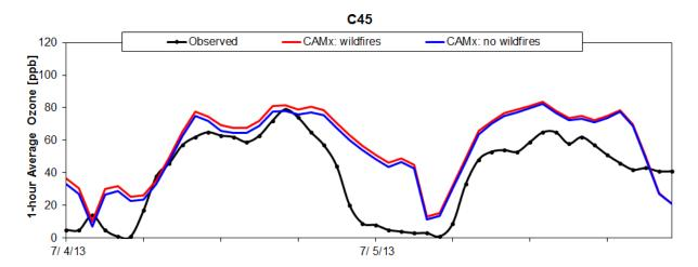
Figure 6-27. Seabrook observed 1-hour ozone (black) versus modeled 1-hour average surface layer ozone for the CAMx run with fire emissions (red) and the CAMx run with no fire emissions (blue).
