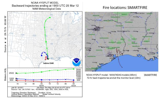
Figure 3-14. March 25 72-hour HYSPLIT back trajectories from Sabine Pass site (left panel) ending at March 25, 2012; SmartFire plot showing fire locations (orange triangles) and 72-hour back trajectories from the BPA site (right panel).
