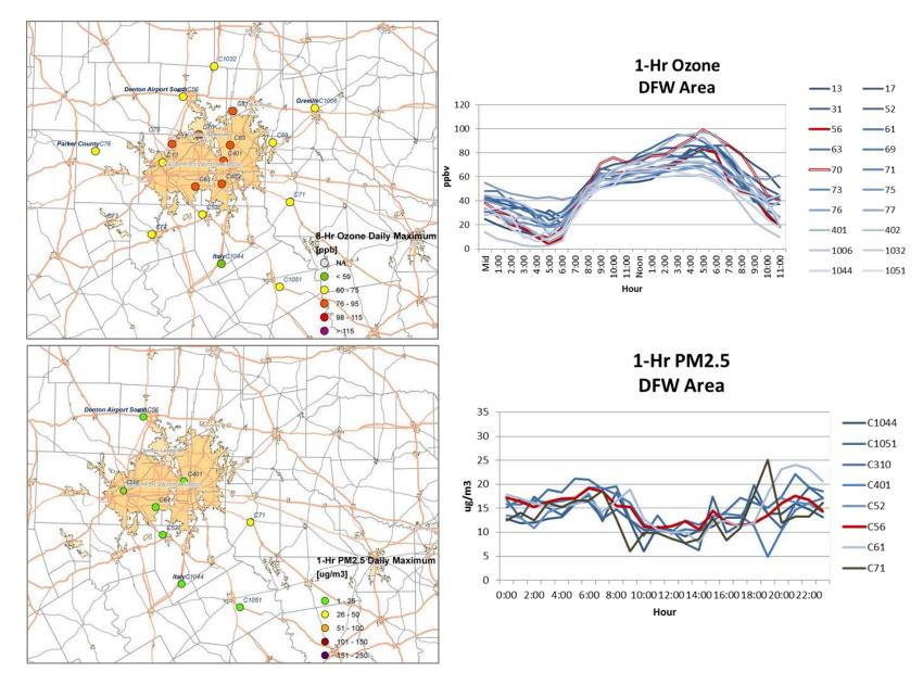
Figure 3-65. June 24 regional ozone (top left and right) and PM<sub>2.5</sub> (bottom left and right) measurements (DFW area time series).
